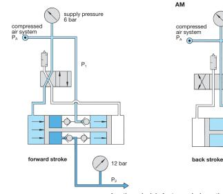
function principle for transmission ratio 1:2
